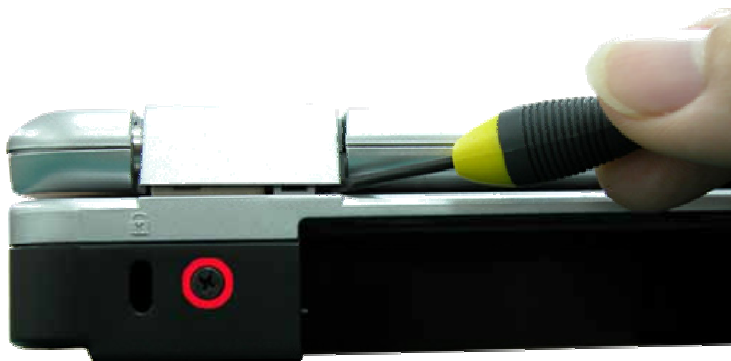
Fig. 17 Removing the top cover screws
